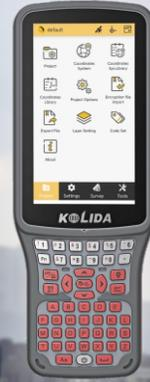
H6 is KOLIDA new generation professional Android controller. It is installed Android 8.1 OS and adopts full keypad with separate keys for 26 letters and numbers makes the input in the field more faster.
