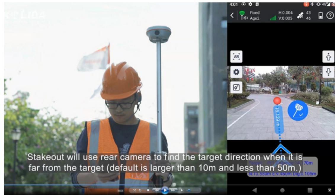
Stakeout will use rear camera to find the target direction when it is far from the target (default is larger than 10m and less than 50m.)
