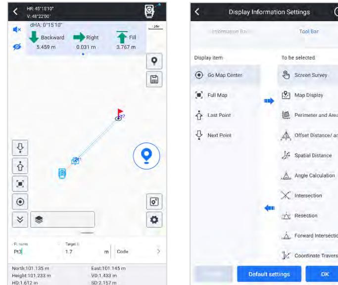
With graphic display, now it is easy to you to observe the relation between occupied point and target points. It will help you to make less mistakes when measuring many points.
